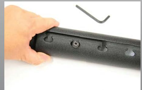
6. Using the small L-shaped wrench insert the smaller headless screws into the sides of the larger pipe (near the top) for additional stability. The screws should be inserted approximately two-thirds of the way into the pipe, as shown:
